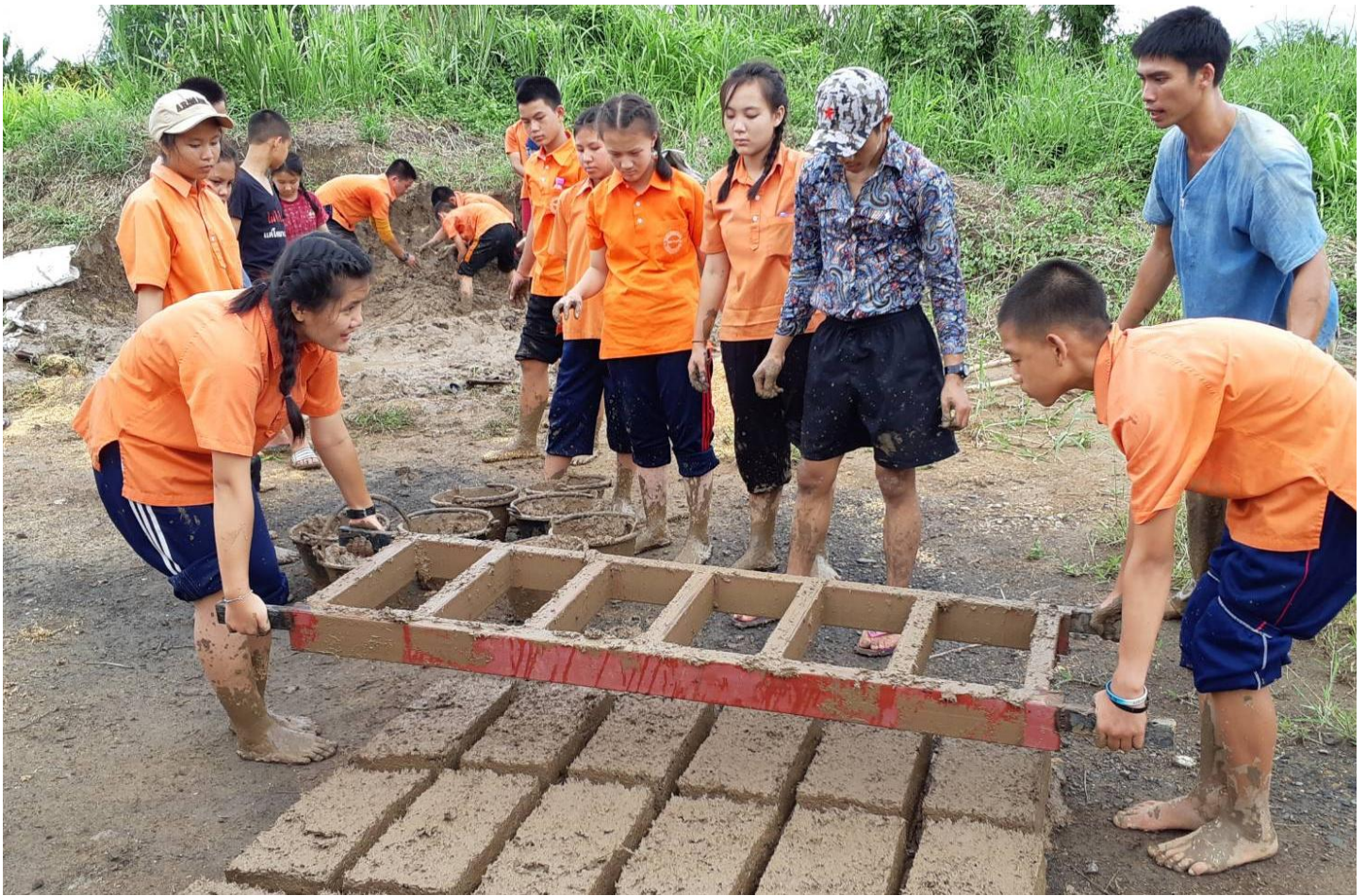
Children making clay-rice husk blocks using molds
